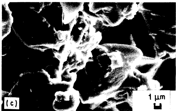
Figure 6 Scanning electron micrographs of the phosphate A23 binder after heat treatments at (a) 500, (b) 800 and (c) 1100 °C (in air).
